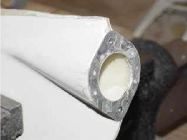
Step 7. You may need to finish up the edges a bit by sanding and using some filler or even a layer of glass to create a nice transition. That is up to you. Except for waiting for the epoxy to dry, doing this only took a couple of hours with minimum hassle.
