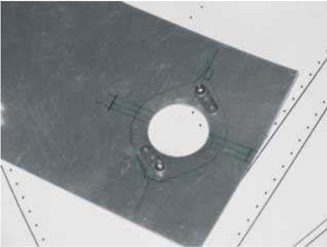
Step 3. Drill holes for the nutplates and cut the plate out of the sheet. Debur and polish it up.
