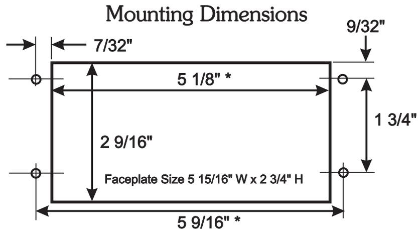
Note: Instruments are 2 3/8" deep. Allow 3/4"-1 1/2" additional depth for connectors on rear of instrument. The warning light requires a 9/16" diameter mounting hole.
